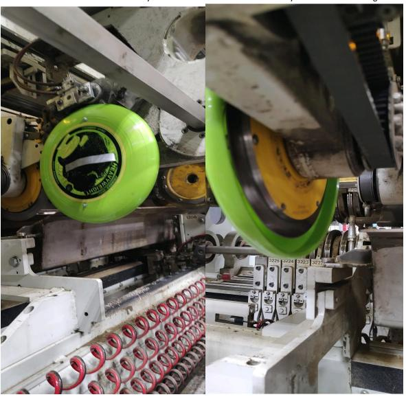
Next step was to find a partner that would help us achieve our goal of a robust guard that is easy to deploy and remove, and that would stand up to the demands of corrugated industry. Over the next three slides you will see the final product of multiple revisions that resulted in an easy to apply/remove, with ergonomic designs including holes to remove slitter blade bolts for change-outs of blades all while minimizing human interface with blades.
